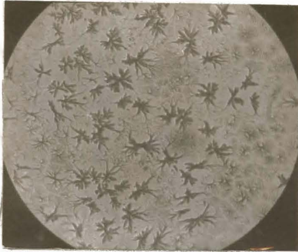
Fig. 1. Crystals of dithizone obtained by evaporating a chloroform solution of dithizone in a small beaker at 50^{\circ}\text{C} . Photographic data: one-half-second exposure, red color filter, magnification 500 x.
