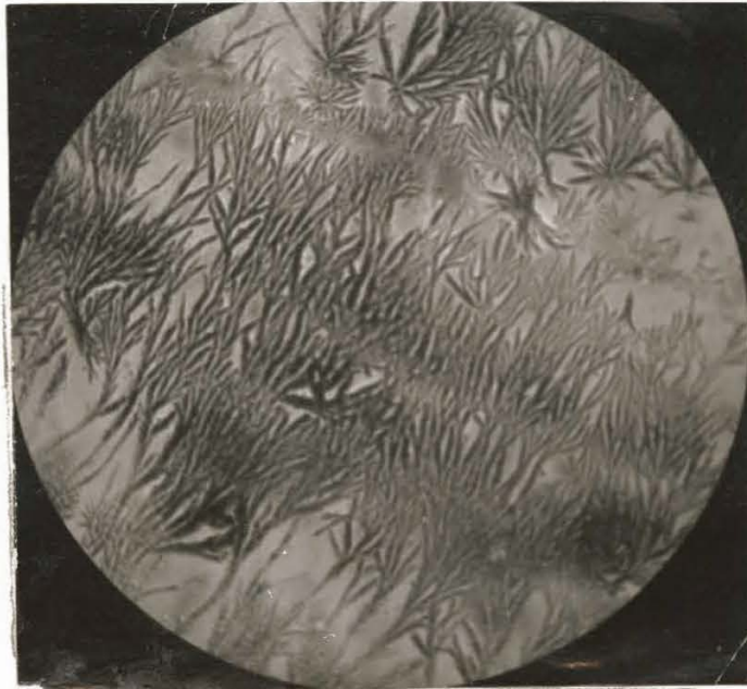
Fig. 2. Crystals of dithizone obtained by evaporating a solution of dithizone on a microscope slide at room temperature. Photographic data: two-second exposure, green color filter, magnification 940 x.
